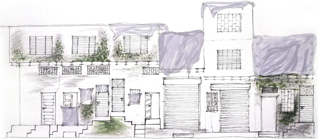
Tarpaulins are easy, quick, and cheap methods of mitigating leakages for the short term
